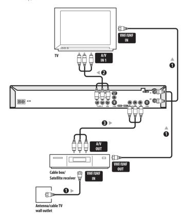
1 Connect the RF antenna cables as shown.
